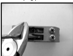
Pull wires tight using a pair of pliers and a vice and screw the wires down on the clamping plate.
